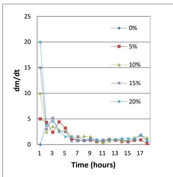
Fig 2d. Drying rate curves for fish at 70°C and varying salt concentration
